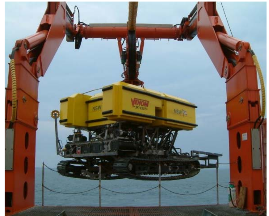
Underwater cable trencher (Chris)
